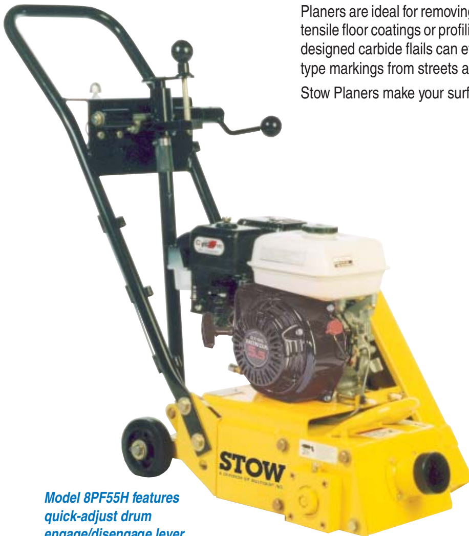
Planer side plate is removable to access flail drum and to mount edger attachment 29021-001.
